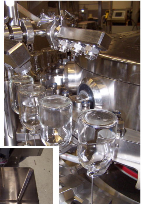
Internal and external container washing.
