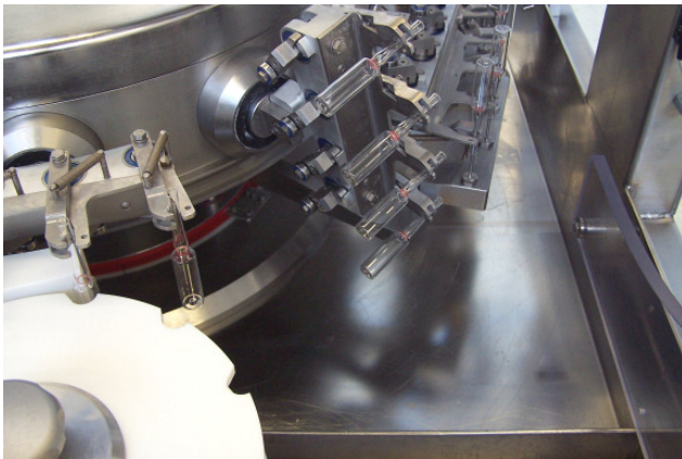
Precise container transfer for unstable containers, including ampoules.
